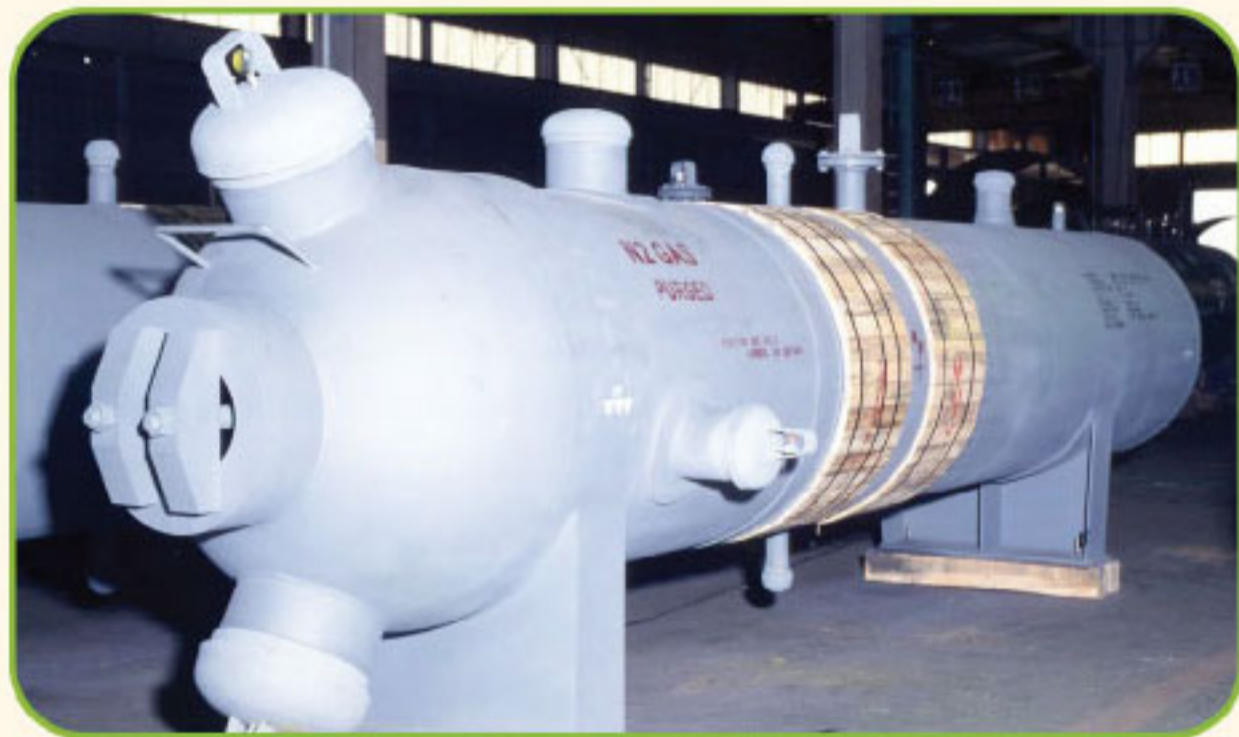
H.P. Feed Water Heater
