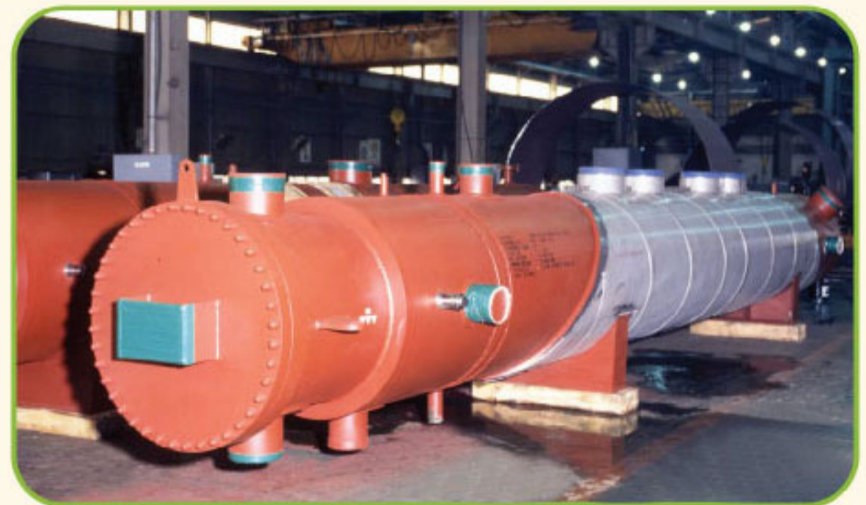
L.P. Feed Water Heater
