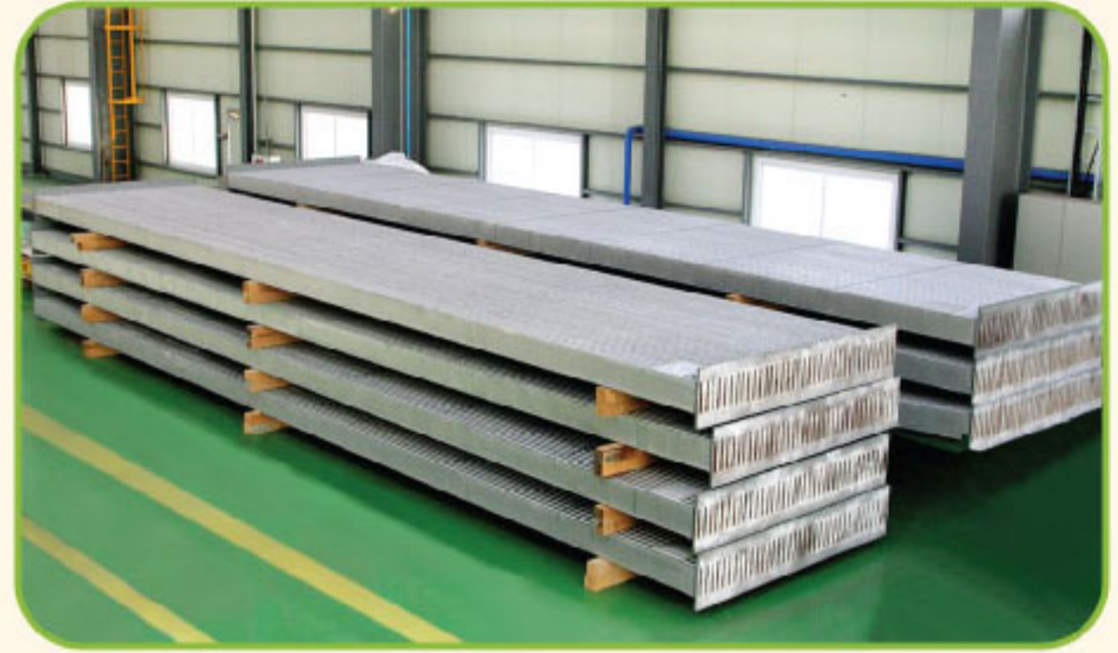
Air Cooled Condenser
