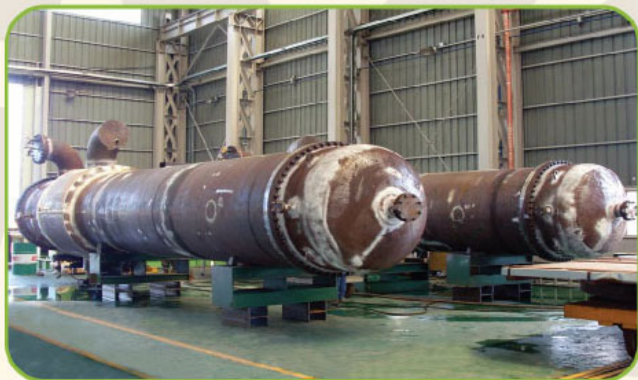
Closed Cooling Water Heat Exchanger
