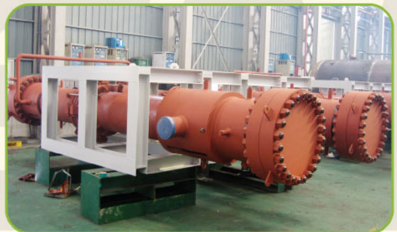
Fuel Gas Heater
